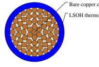
Bare copper conductor LSOH thermosetting insulation
